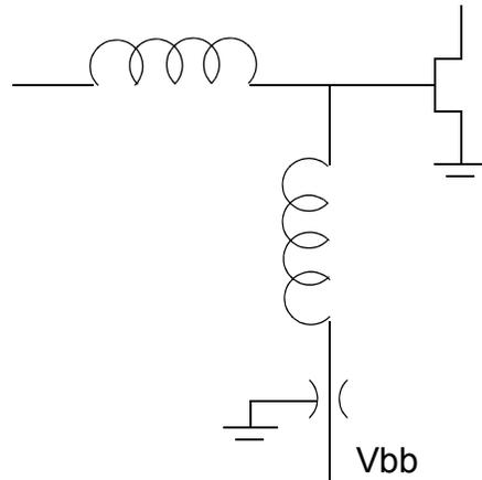
**FIGURE 3. Microwave transistor with input impedance matching**
